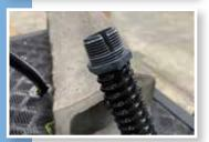
NOTE: The notched end of the hose is designed to attach to the rock and allow passage for a plume lighting cord. If you are installing the fountain without a light kit, simply thread this notched end into the hose union inside the fountain—it will not cause any issues.
