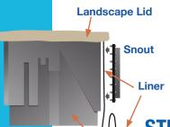
The snout will be secured over the liner before the hole is cut through the liner and excess can be removed.
