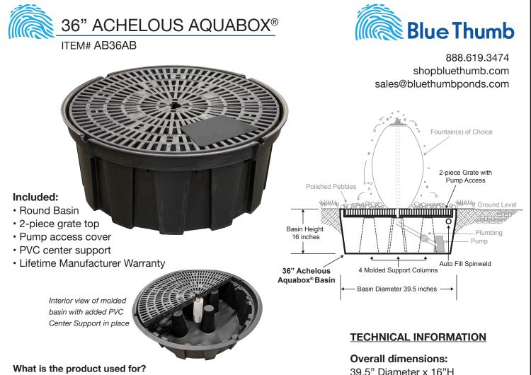
The 36" Achelous AquaBox® is designed as a foundation and reservoir for recirculating water in displays with medium fountains. This basin houses the pump, plumbing, auto fill valve and water reserve.
